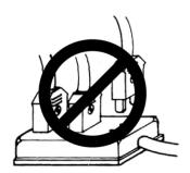
7. Avoid electrical shock when servicing the controller box. (Wait for 6 minutes before opening the cover after turning off the power.)
