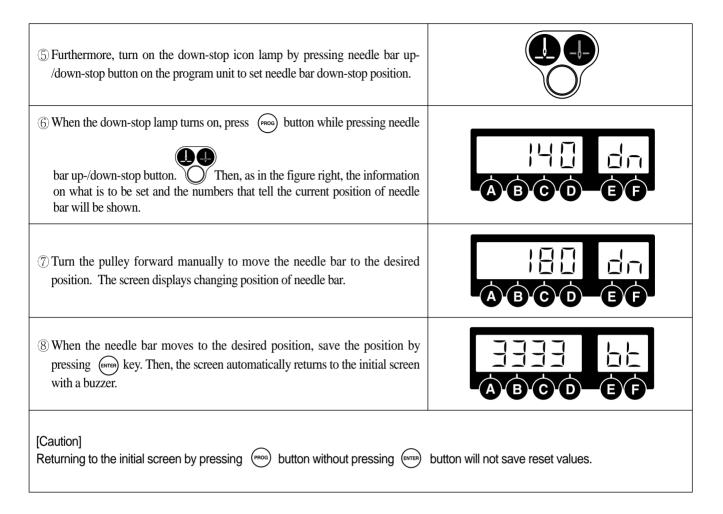
② Setting needle bar up-/down-stop position by using simple controller board (front OP).
