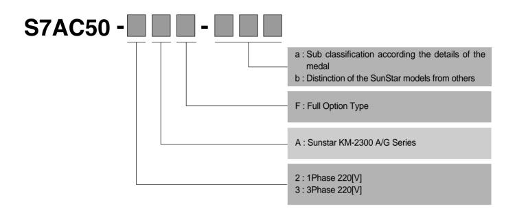
OREDER Ex. S7AC50-2AF refers to SERIES7, 1Phase 220V, FULL FUNCTION CONTROL BOX for normal drop feed.
