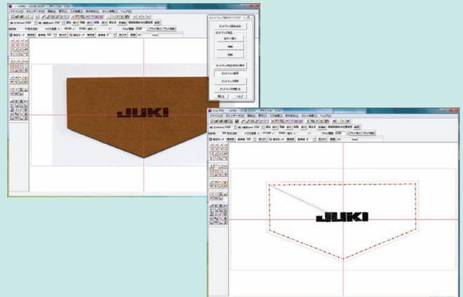
Equipped with template functions that allow to create sewing data easily by input each parameter (For LBH-1790).
