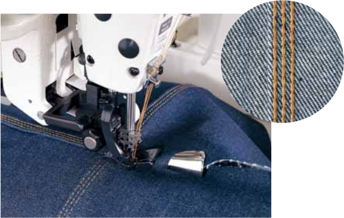
● Beautifully-finished seams are produced by smoothly feeding the overlapped parts of heavy-weight material.
