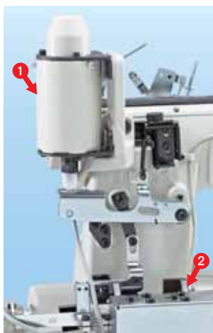
1 Presser lifter drive mechanism 2 Thread trimmer drive mechanism
