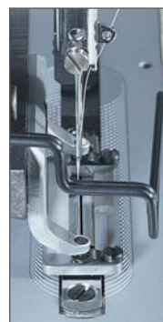
Position of the needle bar during sewing
