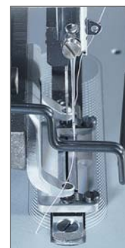
The needle bar can be shifted to the right at the time of threading
