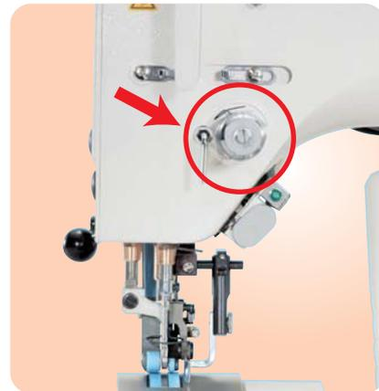
Active tension mechanism
