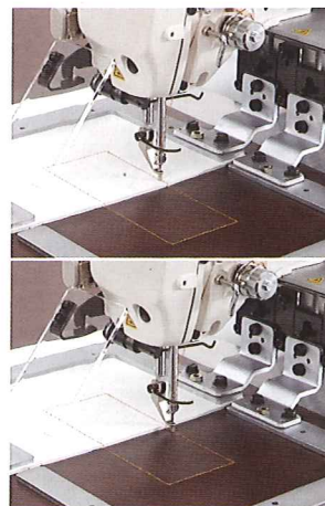
The height of the intermediate presser is constant.
