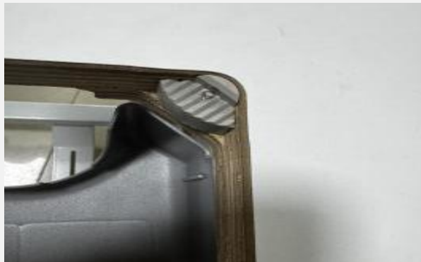
Reinforce the rubber pad of the machine head with nails.
