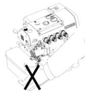
**!** All cords should be secured at least 25 mm away from any moving parts. Furthermore, do not excessively bend the cords or secure them too firmly with staples, otherwise there is the danger that fire or electric shocks could occur.
