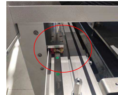
X-axis linear bearing maintenance lubrication
