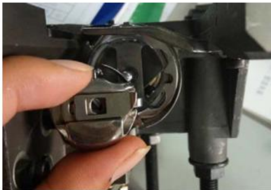
图(Figure)5 准备安装梭壳 Install the rotary hook
