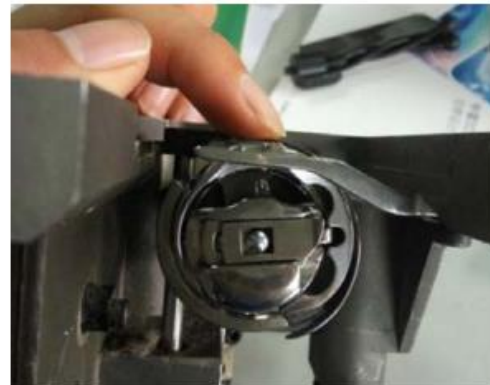
图(Figure)5 准备安装梭壳 Install the rotary hook
