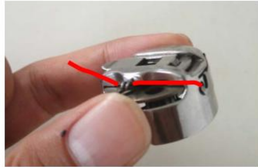
图 (Figure)4 旋梭绕线 the rotary hook winds thread
