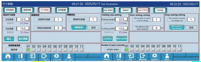
Edge folding height Setting: Set the edge folding width of material. After entering the actual folding width, press the confirm button and the front wheel will automatically move to the set position
