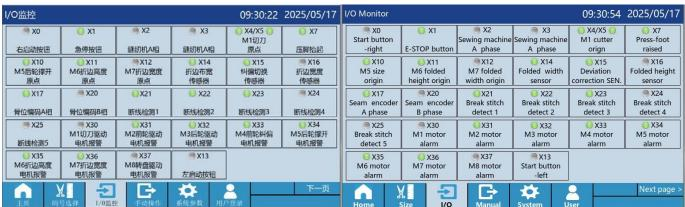
Real-time display of device input and output signal working status, used to detect whether the input signal is abnormal
