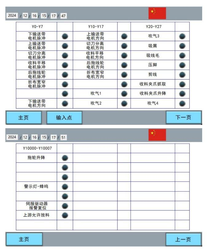
This interface is for all output ports of the device, used to check whether related electrical components and lines are normal.
