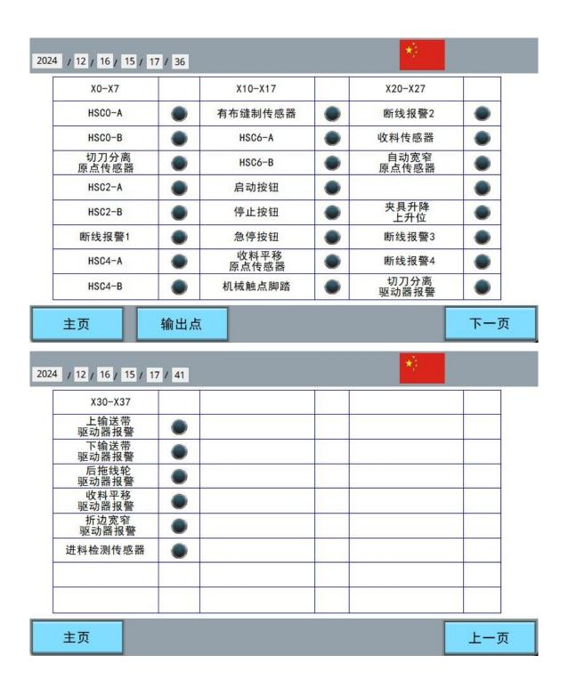
This interface is for all input ports of the device, used to check whether related electrical components and lines are normal.
