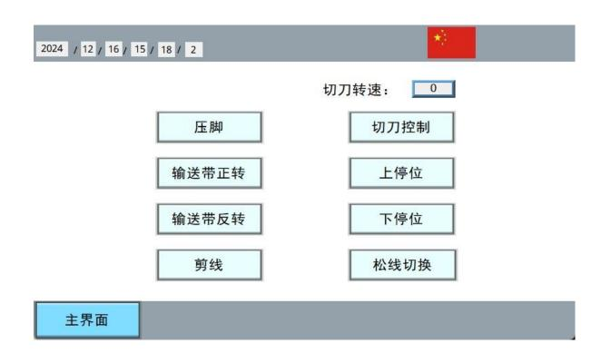
Presser foot: After entering this interface, the presser foot will automatically lift. At this time, it is necessary to ensure that the presser foot is lifted and the cutter is at a low position before pulling the switch of the maintenance equipment. Otherwise, the side-folding width limit plate will be damaged when pulling.
