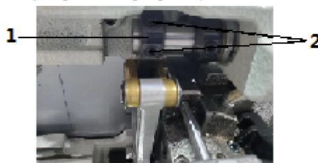
Fig. 54: Adjusting the feed dog height at top dead center
