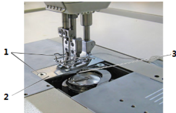
Fig. 36: Assembling and disassembling the throat plate
