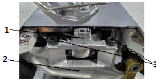
Fig. 37: Assembling and disassembling the feed dog
