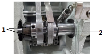
Fig. 57: Adjusting the stroke movement
