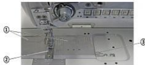
(1) - Throat plate slide (2) - Throat plate (3) - Clamping spring
