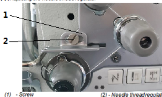
Fig. 77: Adjusting the needle thread regulator
