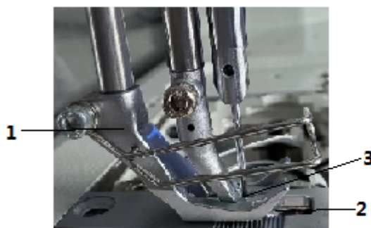
(1) - Walking foot (2) - Feed dog (3) - Needle tip
