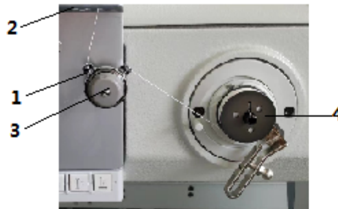
Fig. 17: Winding the hook thread (2)
