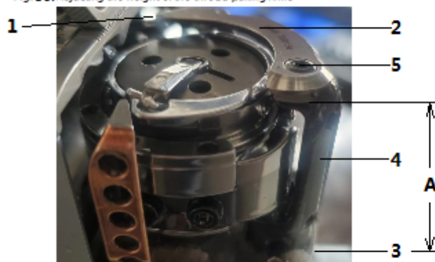
Fig. 86: Adjusting the height of the thread-pulling knife
