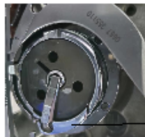
Fig. 26: Setting the hook thread tension
