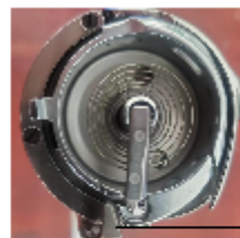
(5) - Screw (6) - Bobbin case lifter
