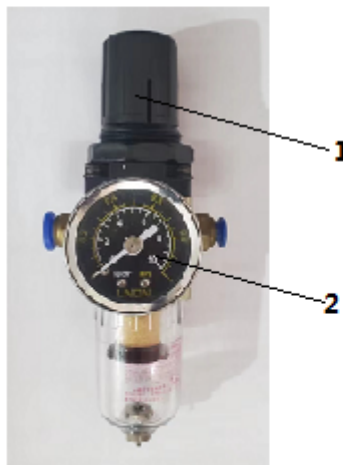
Fig. 5: Setting the operating pressure
