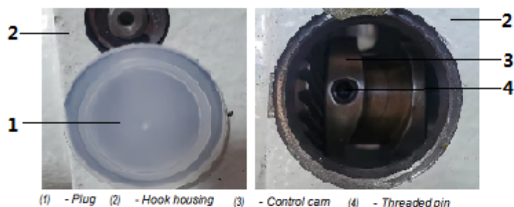
Fig. 70: Adjusting the timing for lifting
