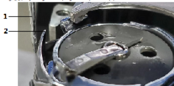
Fig.63: Adjusting the looping stroke position (1)
