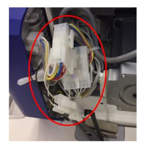
2. Pass the cable of the fan motor component (40230005) through the hole of the table from under the table, and connect the connectors as shown in the figure on the right.
