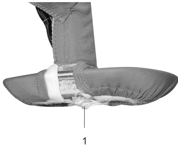
Fig. 25: Replacing the pressing cover (lower buck)
