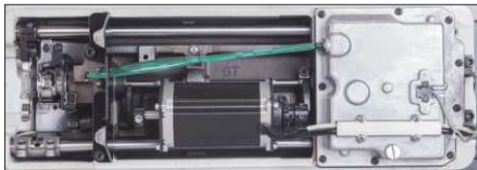
密封油盘，无油无虑 Closed oil pan design
