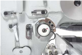
具有断线检测功能 With wire break detection
