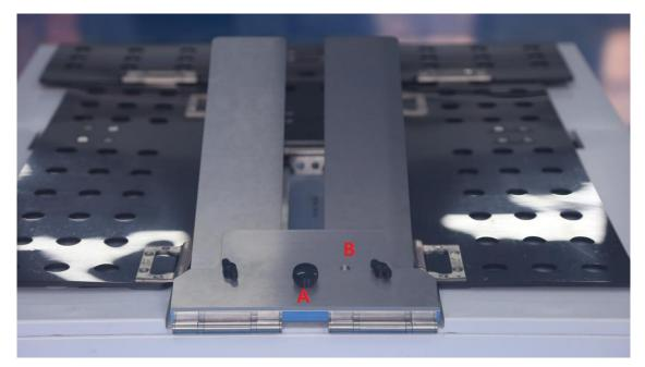
2. When choose "Stack mode", please put the screw in B position to hold the clothes platen in horizontal position as following photo.
