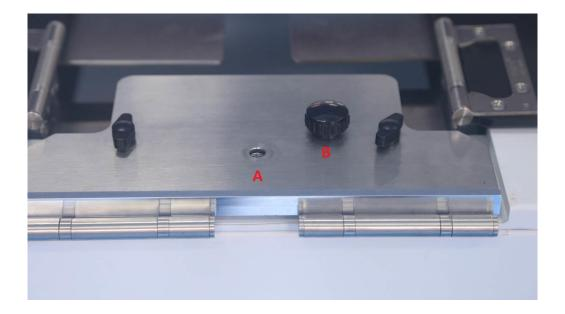
3. Please rotate the handle to adjust the folding width.
