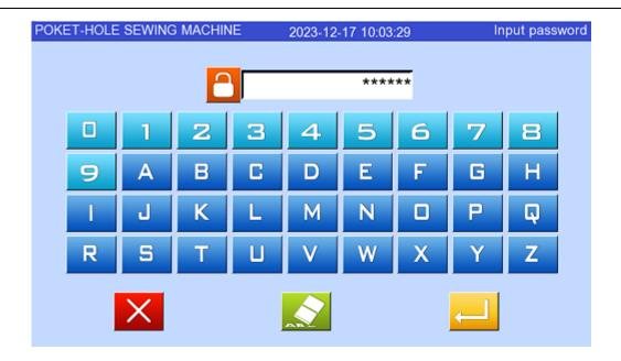
After entering your password, click button, the screen will display: "E1013 controller initialization successful", which means the initialization of the controller is completed. Also initialize the third-level, second-level, and first-level parameters, and then shut down; if the initialization is not successful, prompt, the communication between the screen and the motherboard may have been disconnected, so you need to shut down and restart the computer before initializing it.
