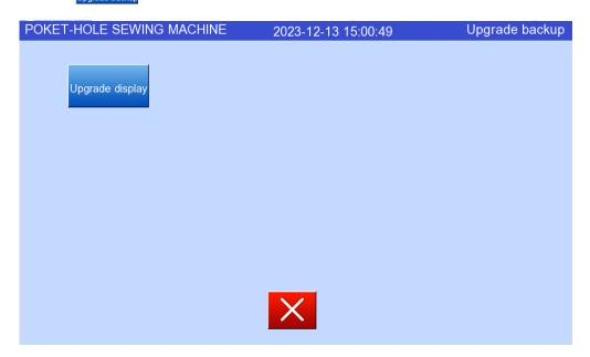
When you plug the USB flash drive into the touch screen USB socket, click button, the system will upgrade your touch screen program to the version number you need. After the upgrade is completed, you will be prompted to turn off the computer and unplug the USB flash drive, and then turn it on again to use the new version...
