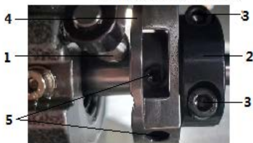
Fig. 87: Adjusting the cutoff curve (1)
