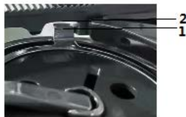
(2) - Slot in the throat plate
