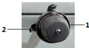
Fig. 85: Adjusting the hook thread guide
