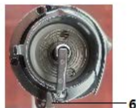
(5) - Screw (6) - Bobbin case lifter
