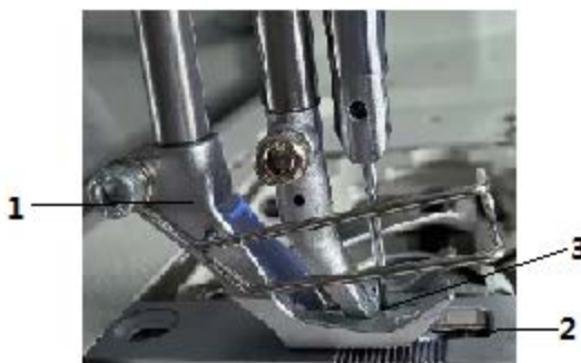
(1) - Walking foot (2) - Feed dog (3) - Needle tip
