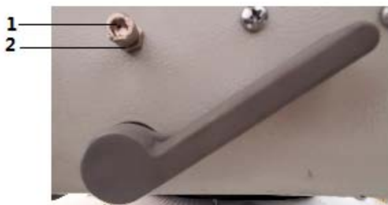
Fig. 76: Adjusting the sewing foot lifting height
