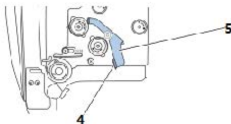
Fig. 24: Setting the needle thread tension (2)
