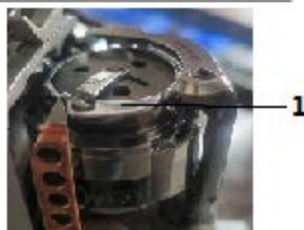
Fig. 26: Setting the hook thread tension
