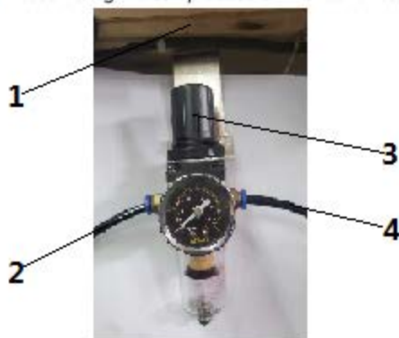
Fig. 4: Assembling the compressed air maintenance unit
