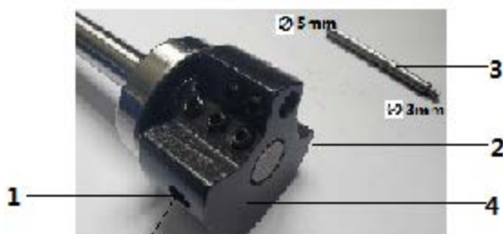
Fig. 39: Locking the machine in place (1)
