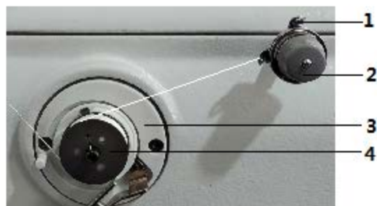
Fig. 17: Winding the hook thread (2)
