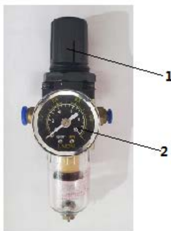
Fig. 5: Setting the operating pressure
