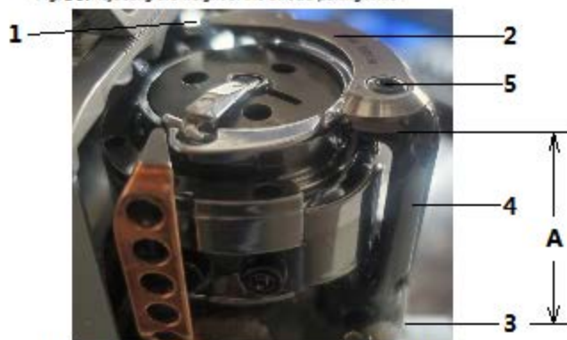
Fig. 86: Adjusting the height of the thread-pulling knife
