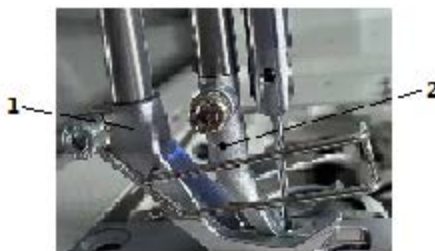
Fig 72: Adjusting an even sewing foot stroke
