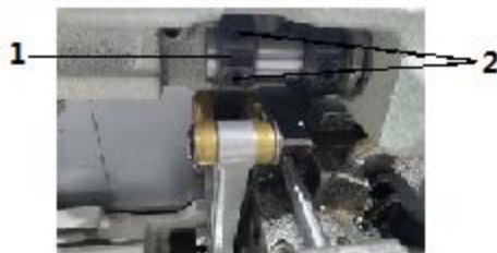
Fig. 54: Adjusting the feed dog height at top dead center
