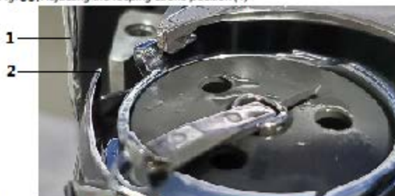
Fig.63: Adjusting the looping stroke position (1)
