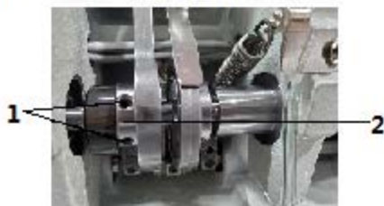
Fig. 57: Adjusting the stroke movement
