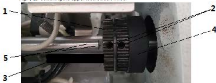
Fig. 44: Positioning the upper toothed belt wheel
