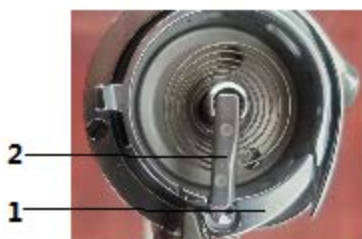
Fig. 67: Adjusting the bobbin case lifter
