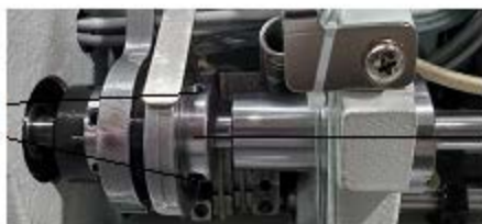
(1) - Threaded pins (2) - Pusher eccentric (3) - Stitch regulator
