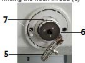
Fig. 18: Winding the hook thread (3)
