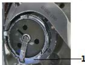
Fig. 26: Setting the hook thread tension
