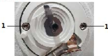
Fig. 84: Adjusting the winder (5)
