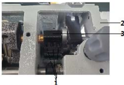
Fig.43: Positioning the arm shaft
