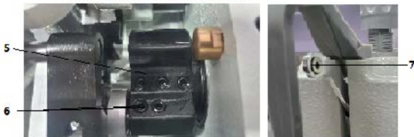
Fig 60: Aligning the needle bar linkage sideways (2)
