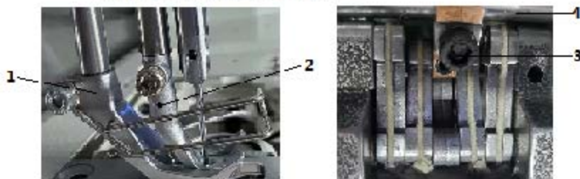
Fig 72: Adjusting an even sewing foot stroke
