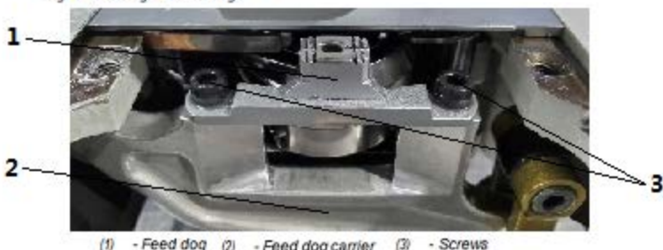
Fig. 51: Moving the feed dog
