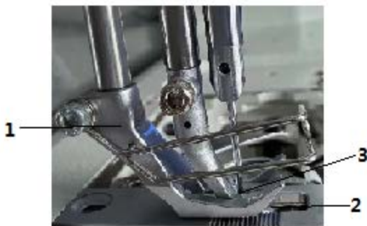
(1) - Walking foot (2) - Feed dog (3) - Needle tip
