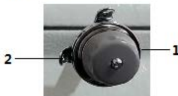
Fig. 85: Adjusting the hook thread guide
