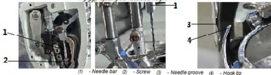
Fig. 66: Adjusting the needle bar height
