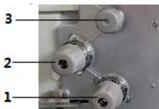
Fig.23: Setting the needle thread tension (1)
