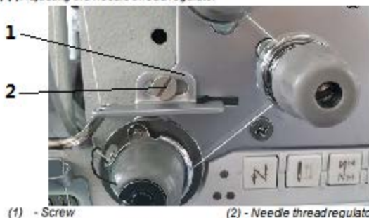
Fig.77: Adjusting the needle thread regulator
