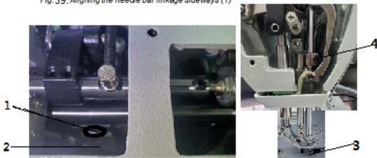
Fig.59: Aligning the needle bar linkage sideways (1)
