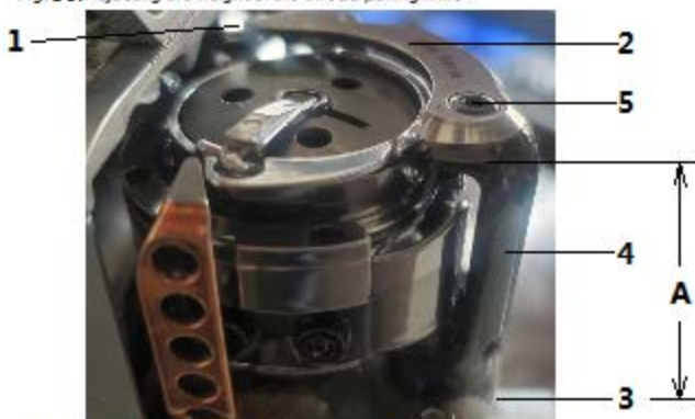
Fig. 86: Adjusting the height of the thread-pulling knife
