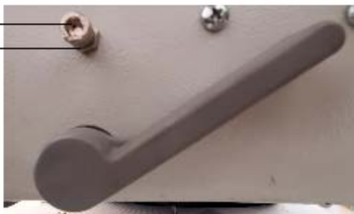
Fig. 76: Adjusting the sewing foot lifting height
