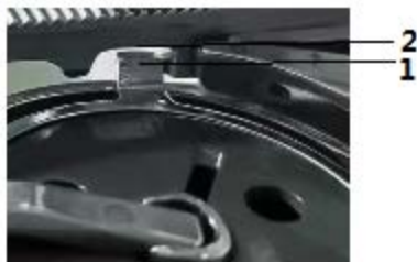
(2) - Slot in the throat plate
