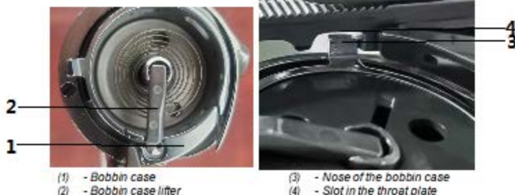
Fig. 67: Adjusting the bobbin case lifter
