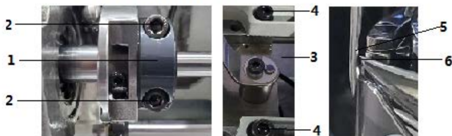
Fig.62: Adjusting the hook side clearance
