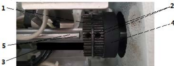
Fig. 44: Positioning the upper toothed belt wheel
