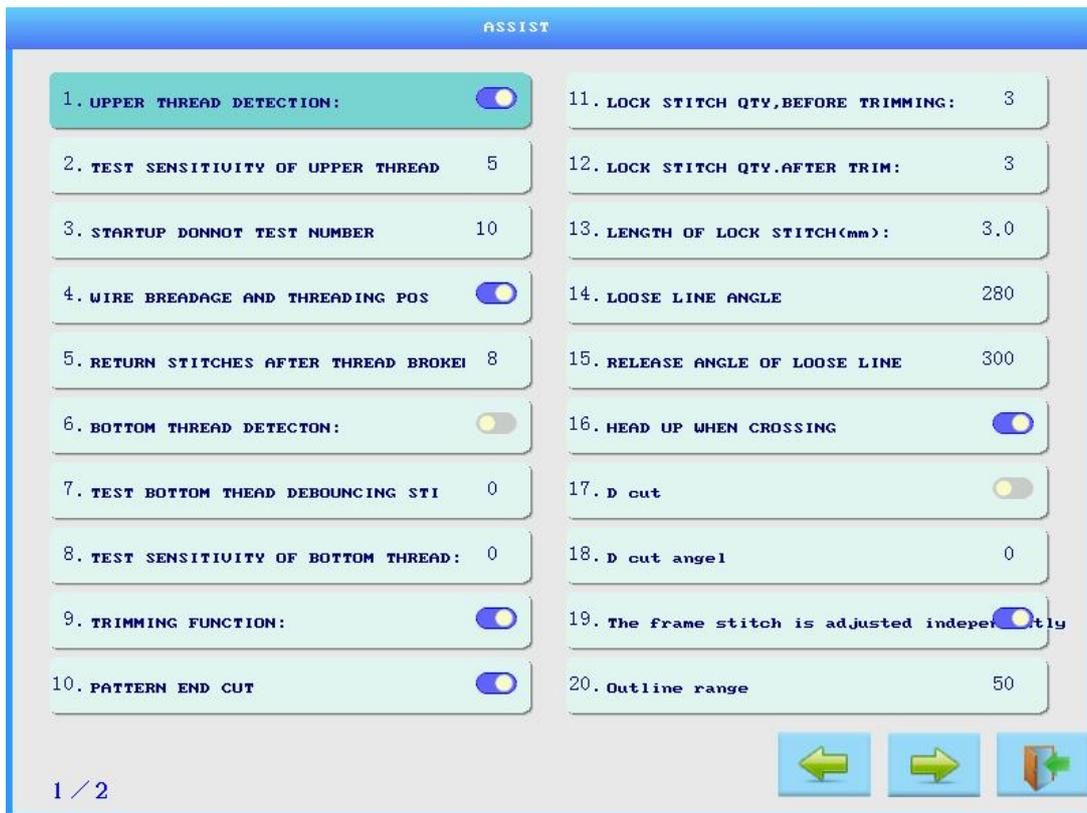
\*[Upper Thread Detection]: Detect broken wire signal, when open will detect broken wire signal, when closed will not detect broken wire signal.
