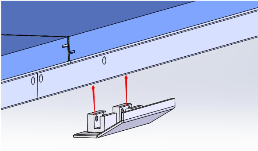
Select the appropriate position at the starting point and the end point of the trip, and adjust to the triggering limit state
