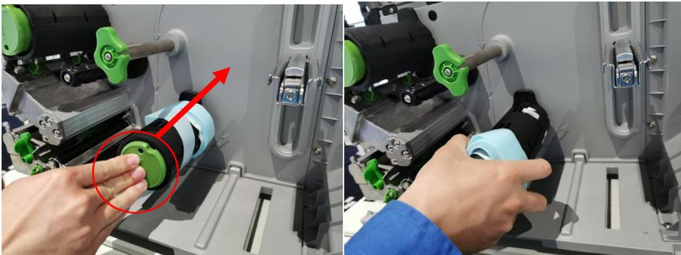
While pressing the green button, remove the loose label roll
