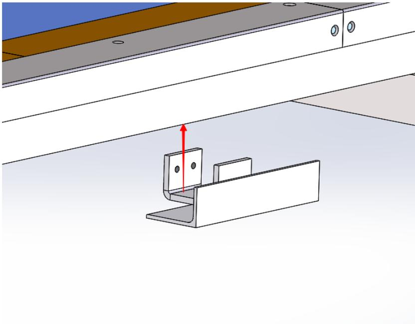
Select the appropriate position at the starting point and the end point of the trip, and adjust to the triggering limit state
