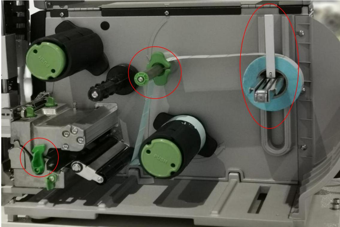
Turn the green switch back to close the printer head, push back the green dial block, turn the block up and attach the label paper roll.
