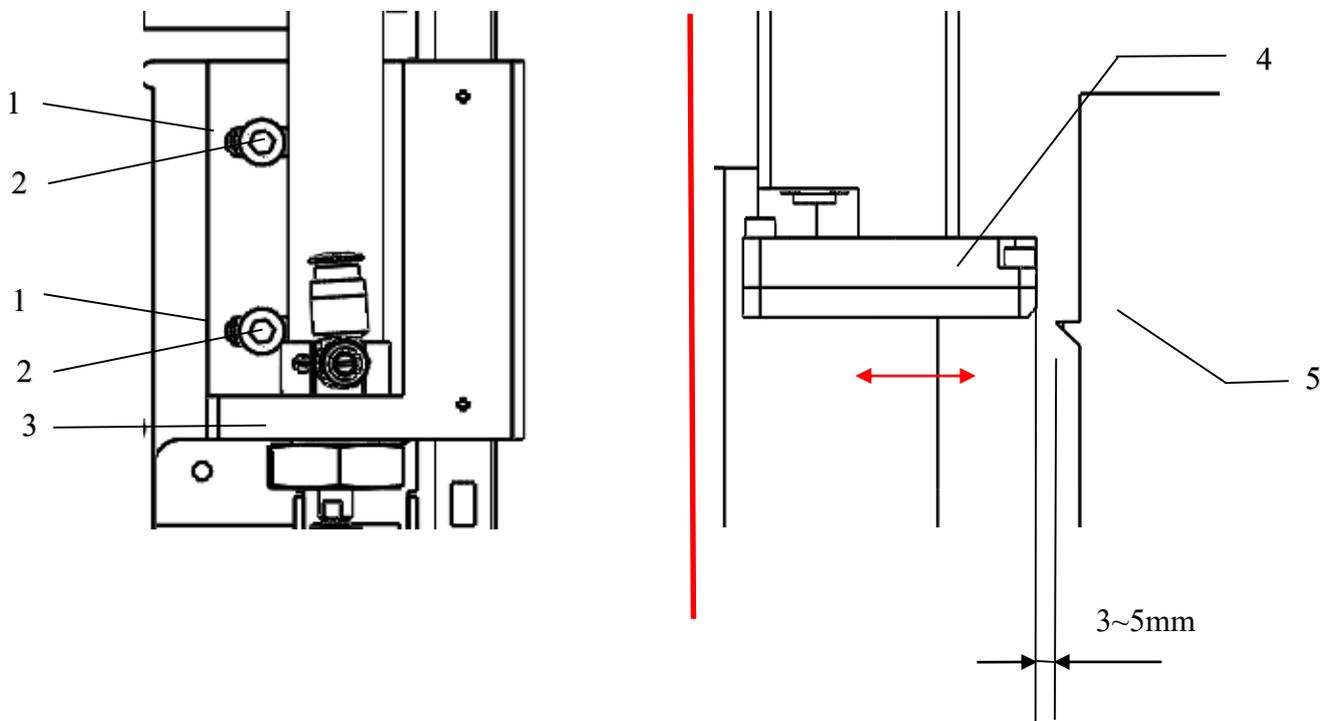
In order to adjust the distance between the sucking disc (4) and the peeling end for the directing plate (5) of the printer, an appropriate adjustment can be made in the printing direction for the sucking disc.
