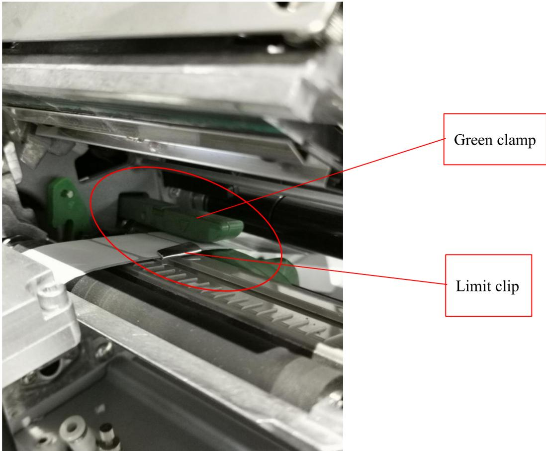
Put the new label paper roll into the position shown, and wrap the label paper back according to the green part of 5.3.1. Note that the label paper passes through the green clamping block at the position shown in the figure, and the label paper is restricted by the limit clip (About to touch the label paper)
