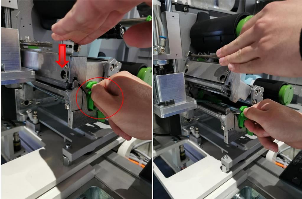
Press one end of the printer down (as in the direction of the arrow), and then turn the green switch back.
