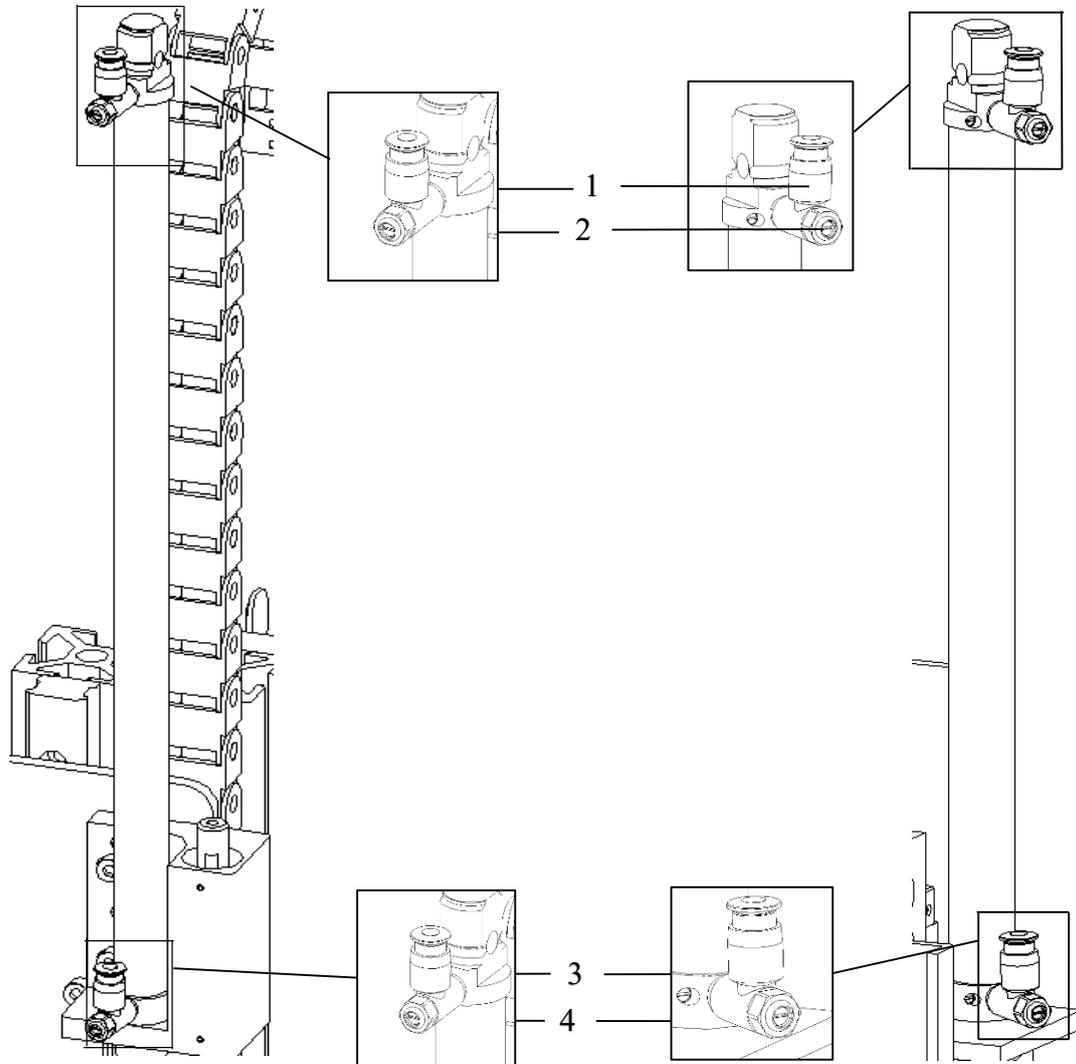
The movement of the cylinder ①, ② can be controlled by the throttles (1, 3) on the cylinder. The two throttles control the up and down speed of the cylinder, which is adjusted by turning the throttles screws (2, 4). The throttles will be turned off by turning it clockwise.
