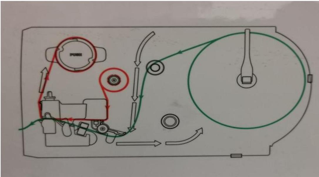
As shown in above picture, the orange one means the install way for TTR, the green one means the install way for temperature-sensitive paper.
