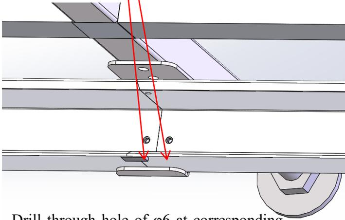
Drill through hole of  $\phi 6$  at corresponding
