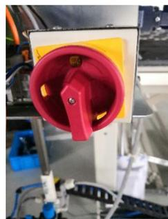
Fig2-12 The CAM Switch
