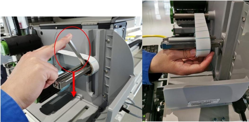
Press the stopper at the label paper down and take out the label paper (the final effect is as shown in the figure above).
