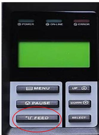
Finally, press the printer FEED key to let the machine adjust the label output.
