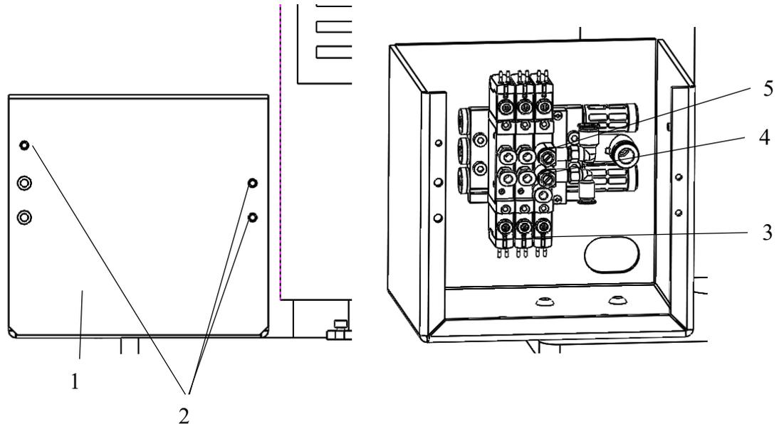
In order to test the labeling function, unscrew the screw (2) in the front of the shell of the valve terminal, then remove the shell (1) to adjust the selector valve conveniently. After remove the shell, the selector valve (3) can be seen, also you can adjust it manually by using tools.
