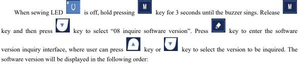
Main control: machine type-MC-manufacturer code-version number
