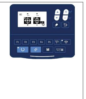
During moving XY motors, if the signal of the origin sensor changes, the icon displayed on the screen will become shadowed.
