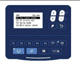
2) Press key to change the function item for test and press key to enter the item for test. The functions represented by each number are as follows:
