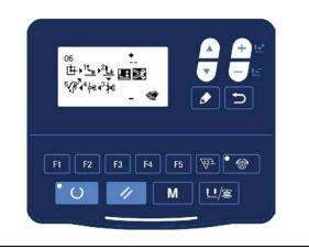
2) Simulation Operation Test of Presser Foot Motor Under this mode, step pedal to level 2 to execute origin search, and then press key to make simulation operation of the motor at various work operation such as lifting up or lowering down.
