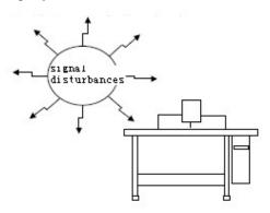
9. If user needs the external signal socket to connect the attachments, the connecting wire shall be as short as possible. The long cable may cause the wrong operation. And the connection cable shall be the isolated cable
