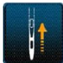
缝制确认键。点击此键，**主轴电机及摆针电机**将找原点，之后系统将进入缝制模式。 Sewing confirmation key. Click this key, the spindle motor and the pendulum motor will find the origin point, and the system will enter the sewing mode.
