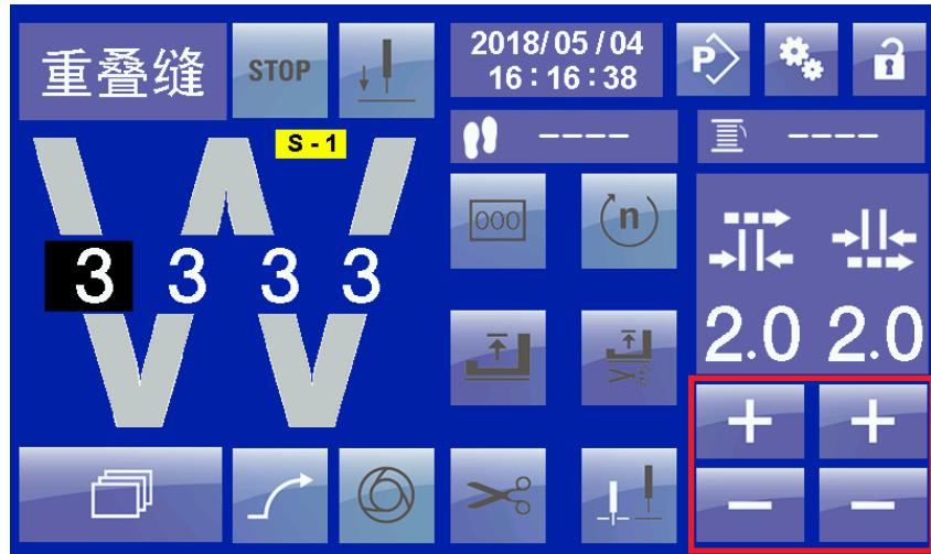
图9 重叠缝界面-滚轮值设置 overlapping sewing interface - scroll value setting
