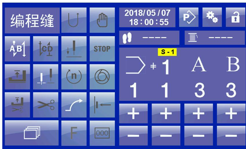
图 12 编程缝界面-设置前加固 programmed sewing interface- setting start back-tacking
