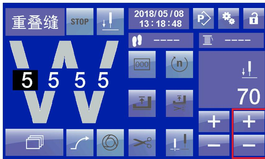
图 10 重叠缝界面-定针设置 Overlapping sewing interface-needle position setting
