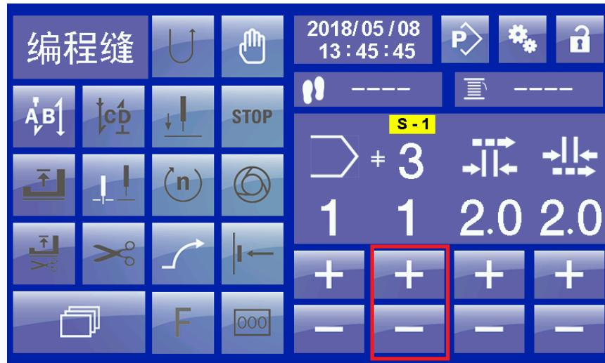
图 10 编程缝界面-多段切换 Programmed sewing interface - multi-segment shift
