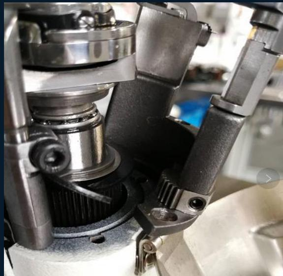
**Step 2:** Install the movable knife holder. The clearance between the movable knife swing gear and the rotary hook outer shaft gear is  $\leq 0.1\text{mm}$ , and it can swing freely without any stuck points.
