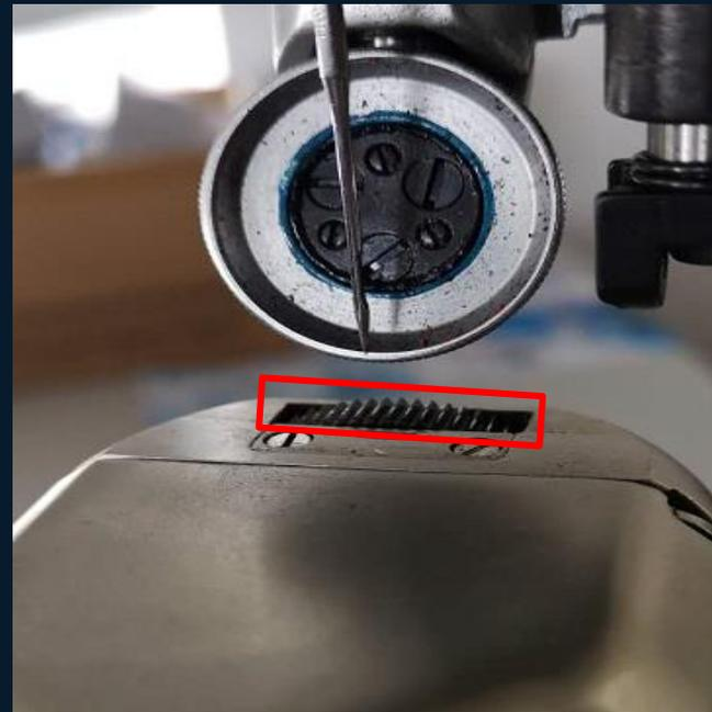
**Figure 2: The teeth of the feeding wheel are 0.8-1.0mm higher than the needle plate; for ultra-thin leather, the teeth of the feeding wheel are 0.3-0.5mm higher than the needle plate.**
