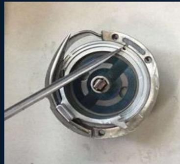
**Step 4: Install the rotary hook and tighten the screws.**
