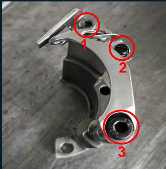
**1** Fixed knife adjustment fixing screw, **2** Clamping piece clamping force adjustment fixing screw, **3** Moving knife fixing screw.
