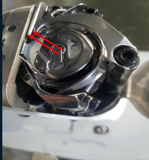
**Step 5:** When the movable knife is at the thread trimming position, the amount of engagement between the movable knife tip and the fixed knife edge is 2-3mm.
