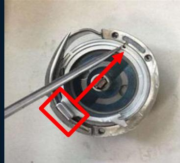
**Step 3: Install the oil supply hole gasket.**
