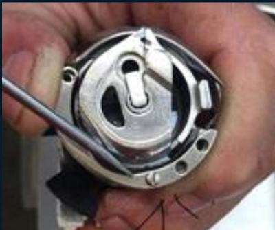
**Step 5: Position the shuttle bladder at the position of the groove on the opposite side of the iron to the groove of the rotary hook, and put the shuttle bladder.**
