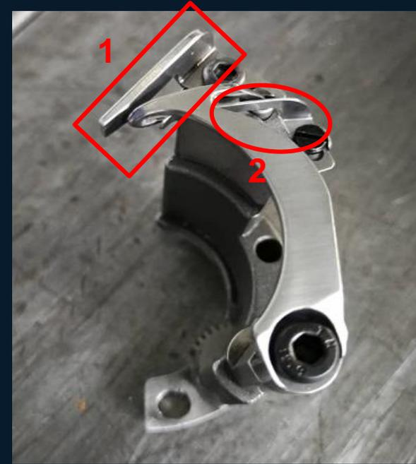
**Step 6:** 1 The moving knife and the fixed knife tangent smoothly, and the pressure is as small as possible to complete the tangent action, and the tangent is neat. 2 The clamping piece is stable and reliable when clamping the wire.
