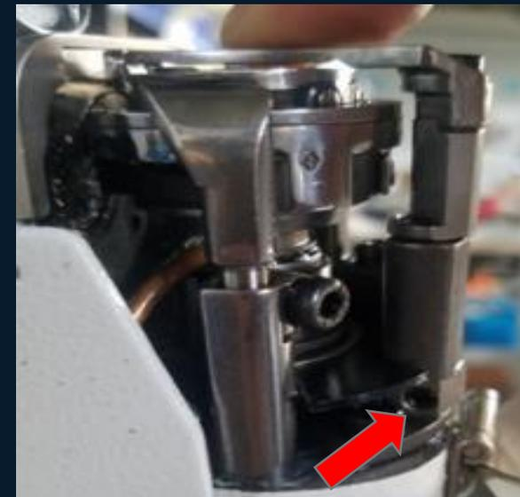
**Step 3:** There are two 2mm screws at the arrow point to adjust the height of the movable knife. The distance between the lower plane of the movable knife and the upper surface of the bobbin case boss is 0.1mm, and the movable knife should not rub against the bobbin case when it moves.
