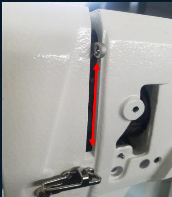
**Step 1: Figure 1** The standard stroke of the thread take-up lever from bottom to top is 62mm.
