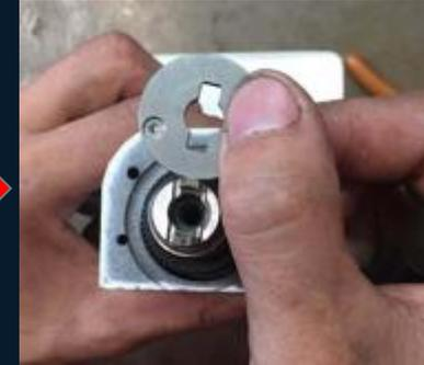
**Step 6: Reinstall the shuttle bladder cover and tighten the 3 screws of the cover.**
