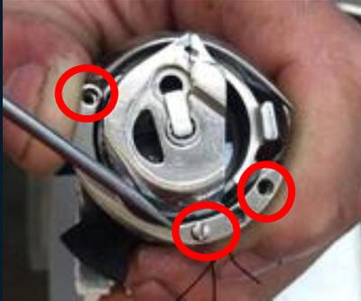
**Step 2: Position the shuttle bladder between the groove on the opposite side of the iron and the groove on the hook, and take out the shuttle bladder.**
