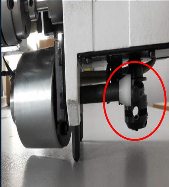
Figure 1 Automatic presser foot lifting electromagnet installation, the distance between the solenoid plunger and the presser foot lifter is 1mm. The upper hole is for the automatic presser foot lifter, and the lower hole is for the knee lifter presser foot lifter.
