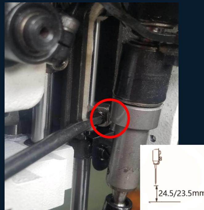
**Step 3: The height of the needle bar can be determined by loosening the screw in Figure 3, moving the needle bar up and down and then tightening the screw. The distance between the single needle and the double needle from the needle plate is 24.5 and 23.5mm respectively.**
