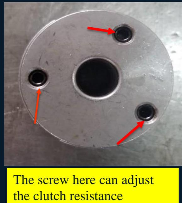
**Step 3: Figure 3** The three screws at the arrow in the figure 3 can adjust the clutch resistance, so that it will not easily get out of position.
