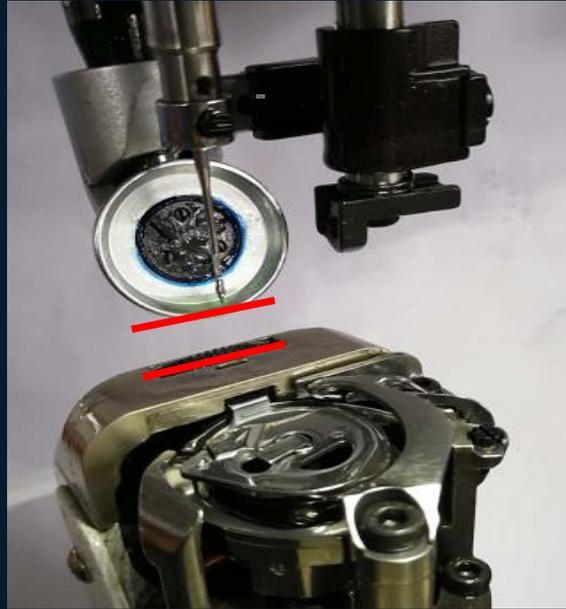
Figure 2 Height of presser foot lift: 6.5mm hand-held, 8.5mm automatic knee-rest 12mm.
