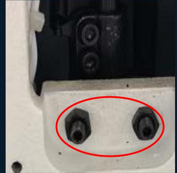
Figure 3 The left side of the adjusting screw for adjusting the height of the presser foot, and the right side is the adjusting screw for the lowest height of the presser foot.
