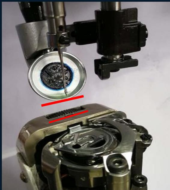
**Step 2:** The distance between the needle tip and the needle plate is 8-12mm as the upper needle stop position. If there is an error, enter the P72 parameter to adjust the upper stop position.
