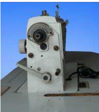
Picture 13 machine head after remove the hand wheel
