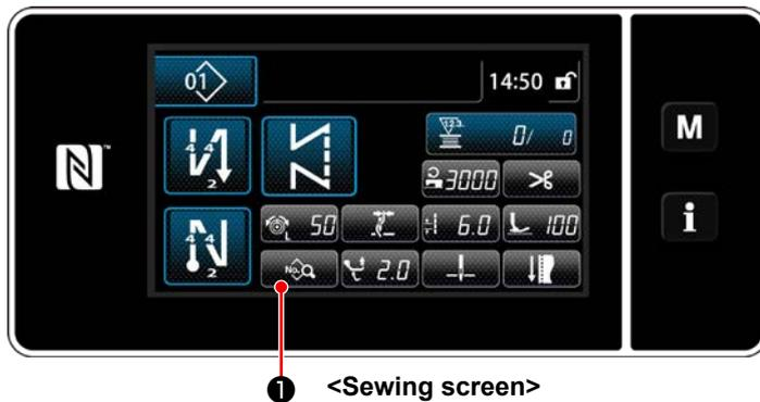
On the sewing screen which is displayed in the case free stitching, constant-dimension sewing or multi-layer stitching is selected, press
