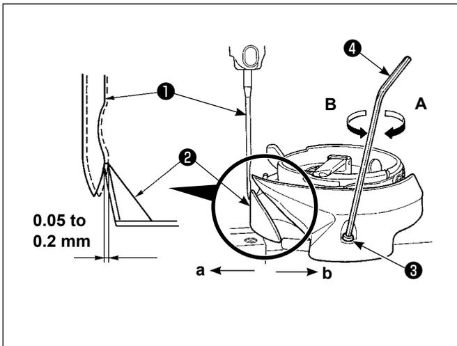
When a hook has been replaced, be sure to check the position of the hook needle guard.
