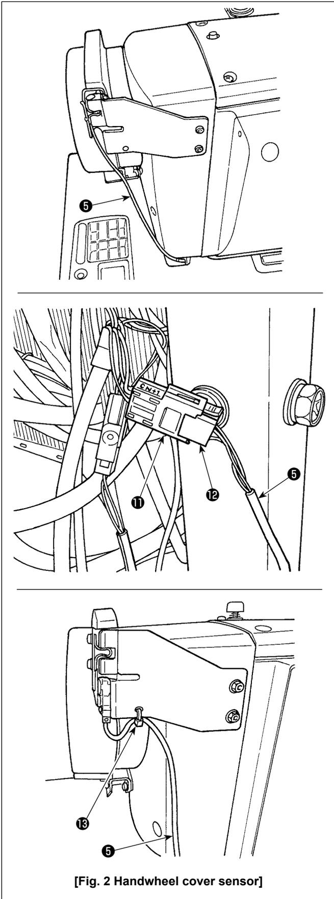
**[Wiring the handwheel cover sensor cord]**
