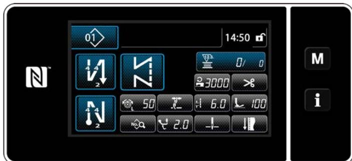
Three different types of the counter are available, i.e., the bobbin thread counter, the sewing counter and the pitch time counter.
