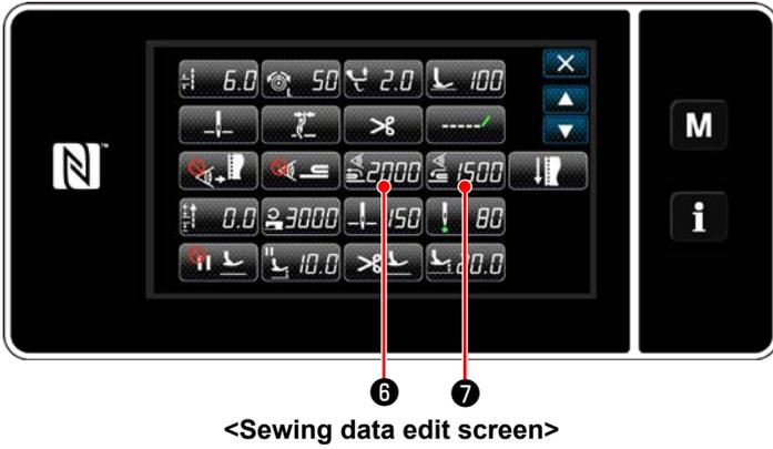
2. Set a "threshold" for the multi-layered section detection.
