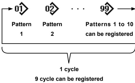
It is possible to combine several different sewing patterns as one cycle pattern for sewing. As many as 10 patterns can be input in one cycle pattern. This function is helpful in the case several different patterns are regularly repeated in a product sewing process. As many as 9 cycle patterns can be registered. Copy the cycle pattern when necessary.
