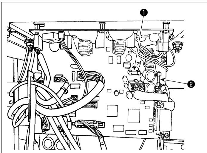
The machine uses the following two fuse.
