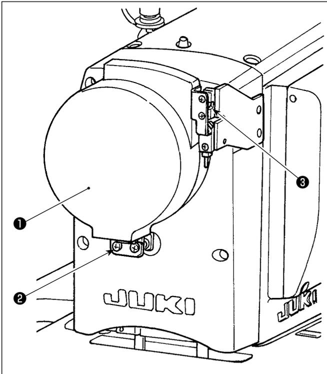
Fix handwheel cover ① with screw ② .
