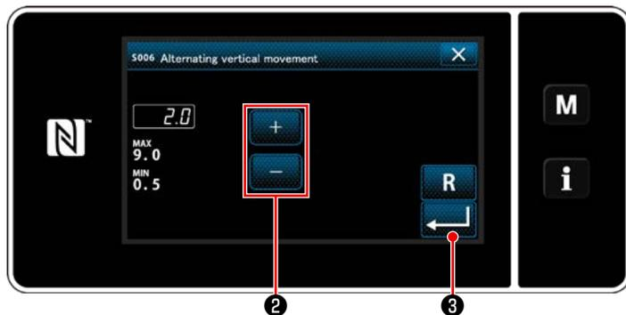
2) Change the alternating vertical movement amount by pressing numeric keypad **2**. (Input unit: 0.5 mm; Input range: 0.5 to 9.0 mm)
