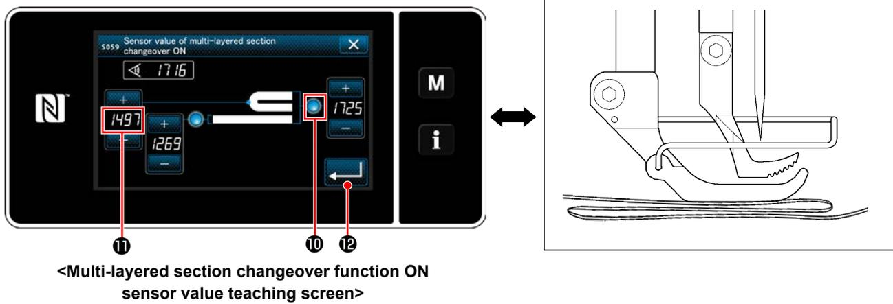
The value of **11** is automatically calculated, and that value becomes the "threshold" for the multi-layered section detection. The value is adjustable with **+** **-** according to the sewing item.
