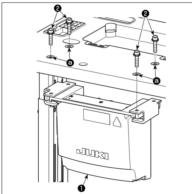
Install electrical box **1** to the table by fixing four accessory bolts **2**, which are supplied with the electrical box, in holes **a** in the table.
