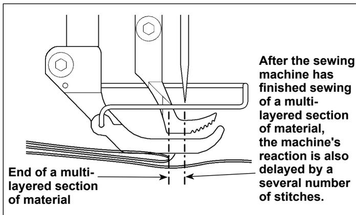
**After the end of multi-layered section of material is fed, the multi-layered section detection function detects the flat section of material to return the sewing conditions to those for the flat section. However, this reaction sometimes delays according to the sewing conditions. If such a delay occurs, it can be corrected by setting the number of stitches of the multi-layered section detection.**
