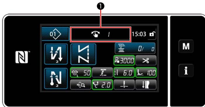
The display of the target data changes and the number (1 to 4) of the one-touch change over function is displayed in ❶ while the one-touch changeover function works.
