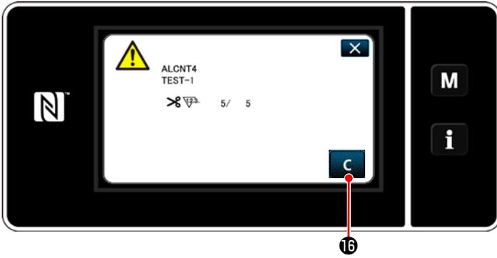
20) When the preset number of counts for the counter is reached, the warning screen is displayed.
