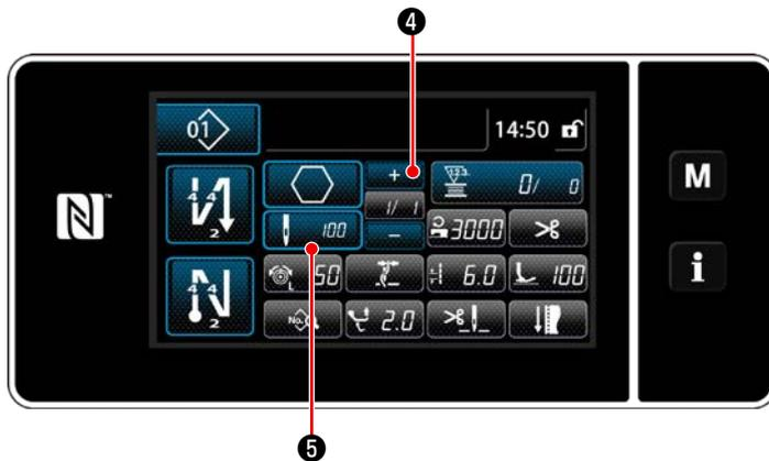
Press **+** ④ to confirm the teaching data on the current step. Press **100** ⑤ to change the current screen to the number of stitches input screen for the next step.
