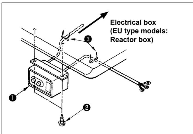
Fix power switch ① under the machine table with wood screws ② .
