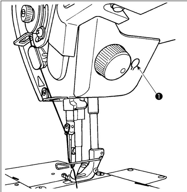
\* This LED is intended to improve operability of the sewing machine and is not intended for maintenance.
