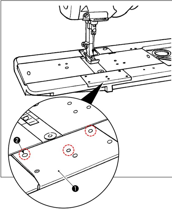
Remove screws ② (three pieces) from front bed slide ① . Install the attachment with those screws.
