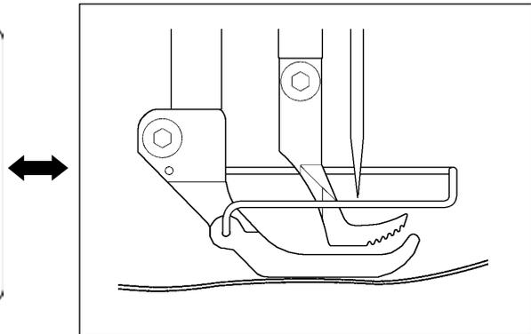
4) Place the multi-layered section of material under the presser foot, and press **10** .
