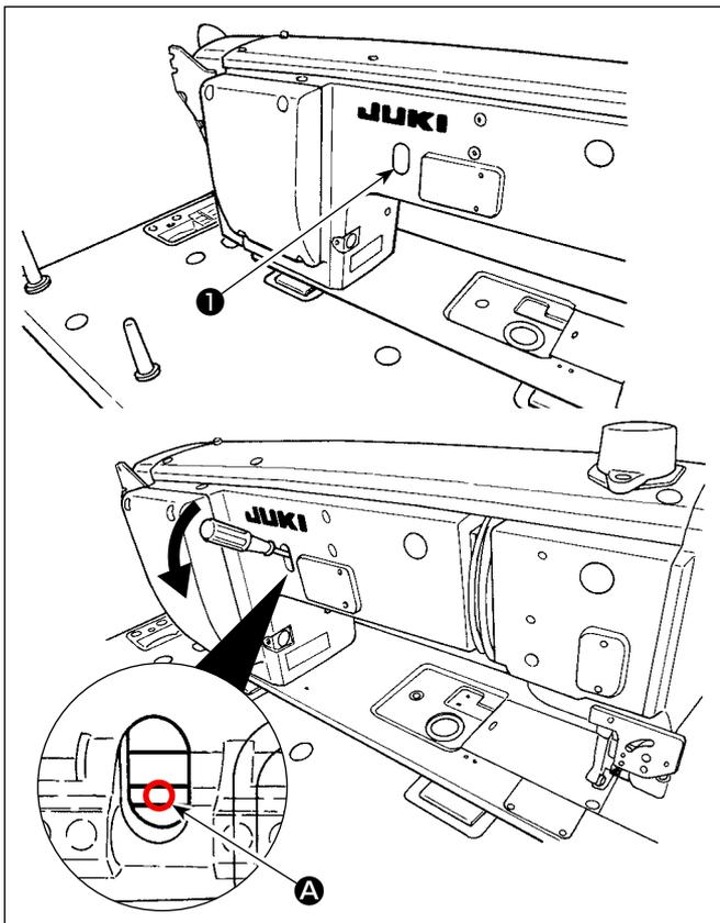
In the case it is necessary to lift the presser foot at a time of emergency such as a power failure, detach rubber cap ❶, put a screwdriver or the like between the shafts and push down the screwdriver to lift the presser foot.
