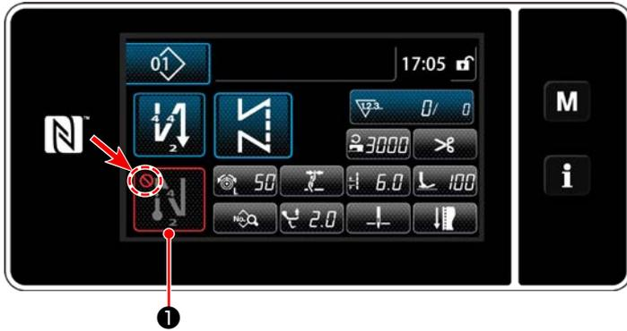
The sewing-end reverse feed stitching pattern can be operated when the sewing-end reverse feed stitching function is placed in the ON state (⊘ mark is not displayed).
