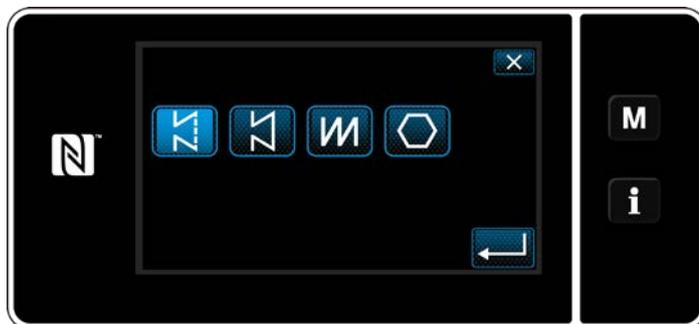
3) Select the desired sewing shape (free stitching, constant-dimension sewing, multi-layer stitching, polygonal shape stitching).
