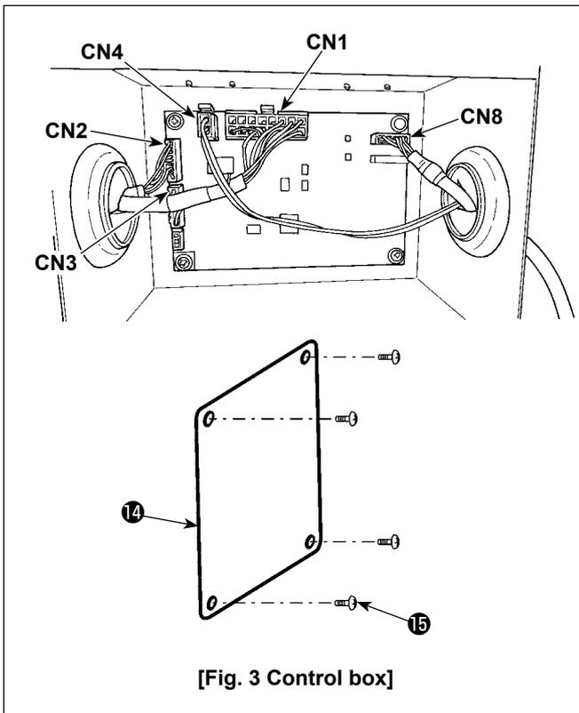
\* Connect the cables to the CN1, CN2 and CN3 while inserting the former through the hole in the left surface of control box. Connect the cables to the CN4 and CN8 while inserting the former through the hole in the right surface of control box.
