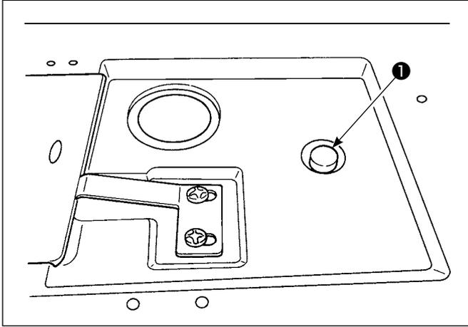
The safety clutch functions when an excessive load is applied to the hook or the other components during sewing. At this time, the hook will never rotate even if turning the handwheel. When the safety clutch has functioned, remove the cause and reset the safety clutch as given in the following procedure.
