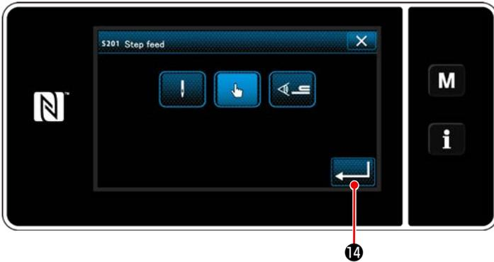
9) When displayed step 13 is pressed, the "step changeover reference selection screen" is displayed.
