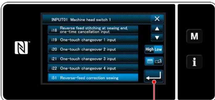
In the case the function item i51 or beyond is selected, the operation to be carried out when the button is pressed is set.
