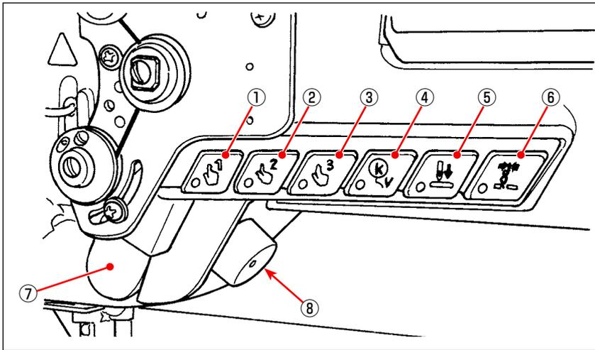
Operations can be assigned to machine head switches ① to ⑥ , hand switch ⑦ and jog dial ⑧ .
