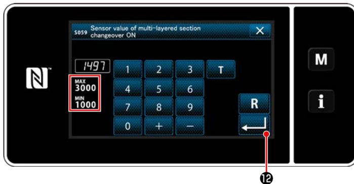
Check that the "threshold" you have set is entered. Then, press **←** **12** again to confirm the setting. Note that the "threshold" can be directly entered or corrected on this screen.
