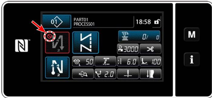
The sewing-start reverse feed stitching pattern can be operated when the sewing-start reverse feed stitching function is placed in the ON state (no mark is not displayed).
