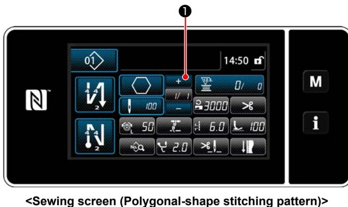
The current step can be changed by pressing
