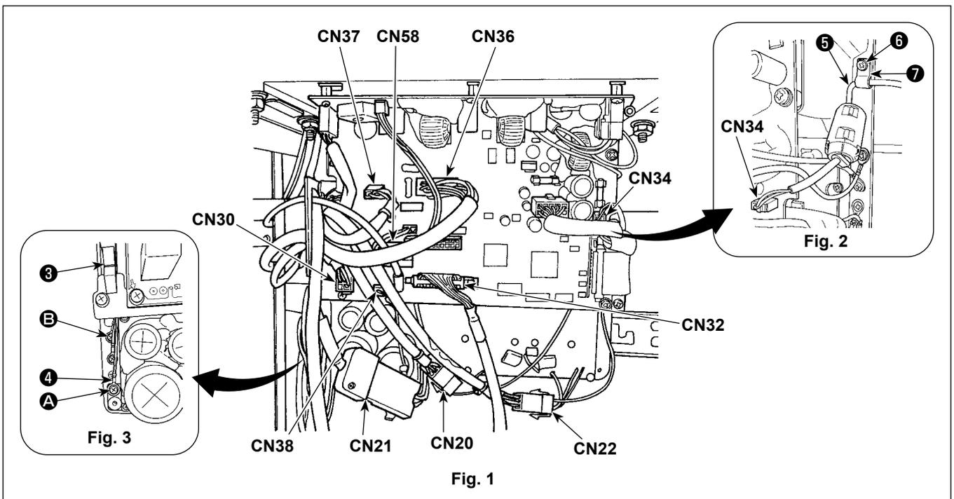
2-14-2. Connection of the cords coming from the stitch skipping detecting device, bobbin-thread remaining amount detecting device and cover sensor
