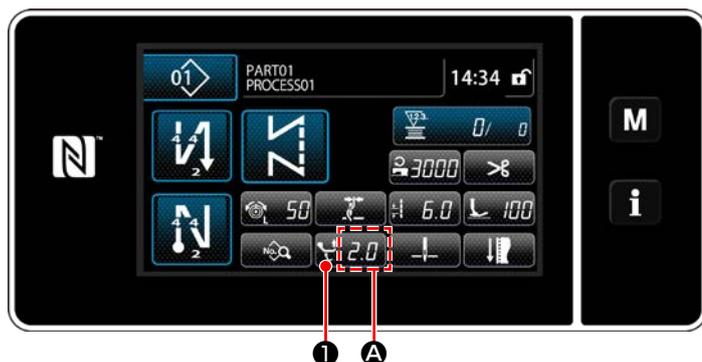
The alternating vertical movement amount is displayed in section **A** on the operation panel.
