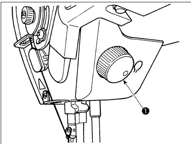
When jog dial ❶ is pressed, the needle up/down correction switch function works. The function of switch can be changed. (Refer to "4-11. Custom switch" p.39)
