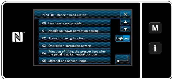
4) Select the function item to be assigned to the switch. Then, select the input signal status ( **High** / **Low** ).
