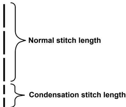
In the case of performing condensation stitching after thread trimming (condensation stitching is placed in ON), set values of the stitch length and that of the number of condensation stitching can be changed.
