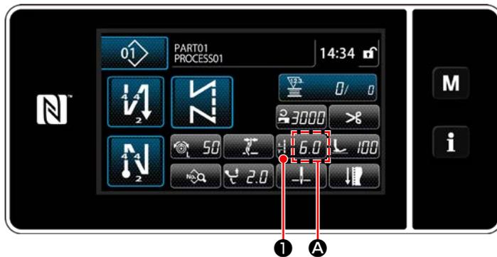
Stitch length is displayed in section **A** on the panel. (Example of display : 6.0 mm)
