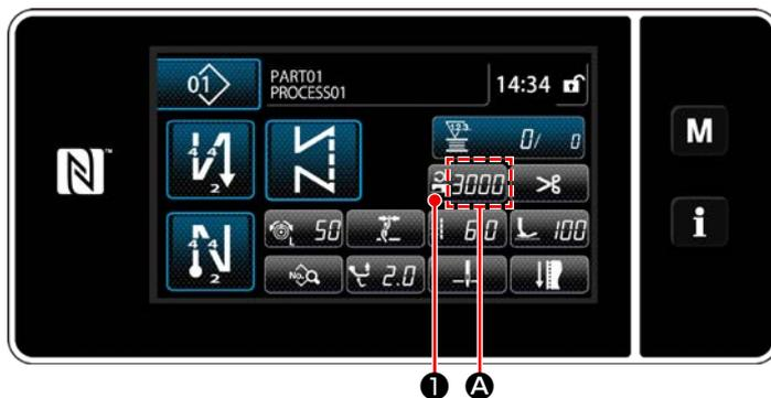
The sewing speed is displayed in section **A** on the panel. (Example of display : 3,000 sti/min)
