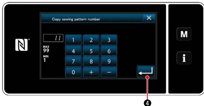
3) Input a copy pattern number with the numeric keypad.
