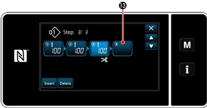
8) In the case a step can be additionally registered to a sewing pattern, step 13 which is not yet set is displayed in the last field.
