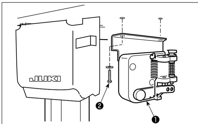
Secure pedal sensor **1** to the table with two plain washers and two wood screws **2** both of which are supplied with the electrical box.
