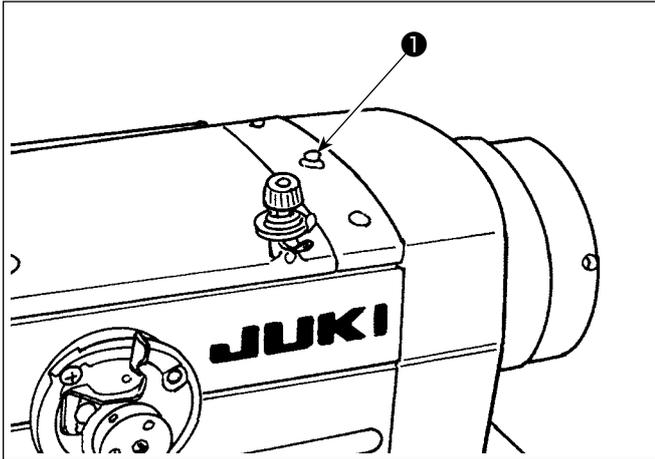
Power lamp ❶ lights up when the power to the sewing machine is turned ON.
