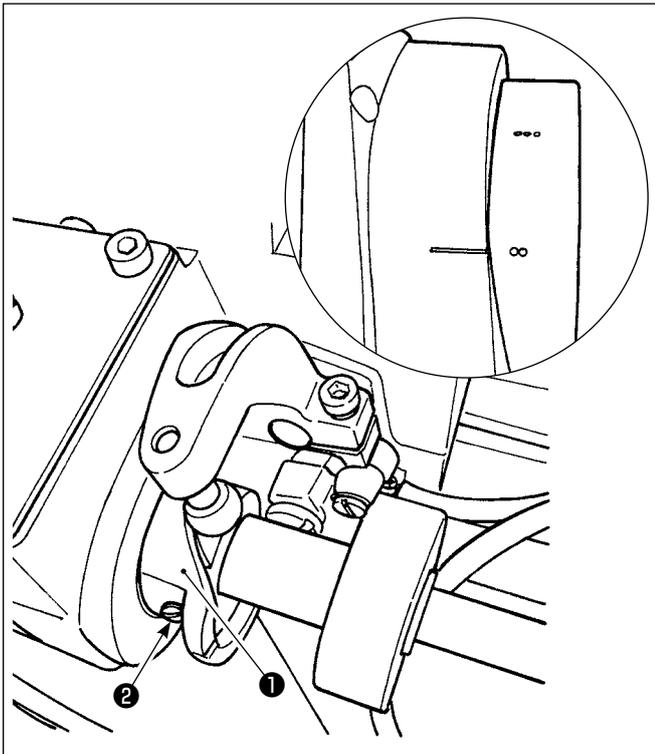
Bring the moving knife to its front end. At this time, position the thread trimming cam so that the two marker dots on the handwheel align with the marker line of the motor cover. Then, tighten thread trimming cam setscrew ② to fix thread trimming cam ① .
