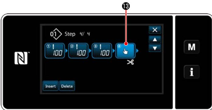
11) When step 13 is pressed again, the "sewing data edit screen" is displayed.
