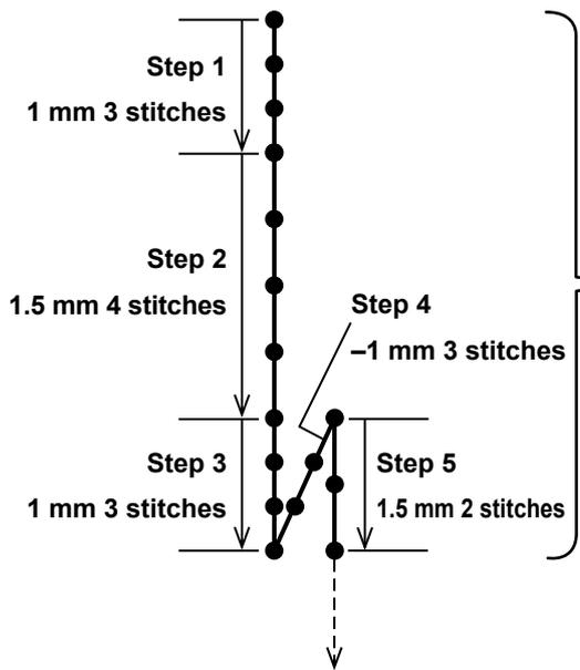
Condensation stitches can be sewn while specifying needle entry points as desired, by setting a condensation custom. As many as 20 steps can be created in one pattern. The maximum number of patterns that can be registered is nine.
