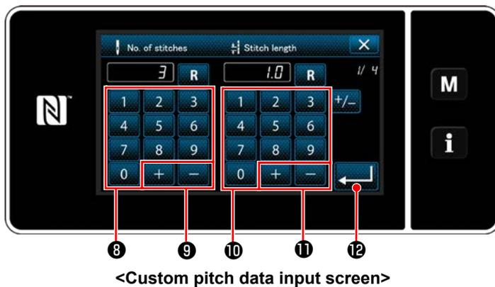
1. In the case of setting the number of stitches Custom pitch pattern input procedure is described as follows using < Figure: Example of the custom pitch > as an example.
