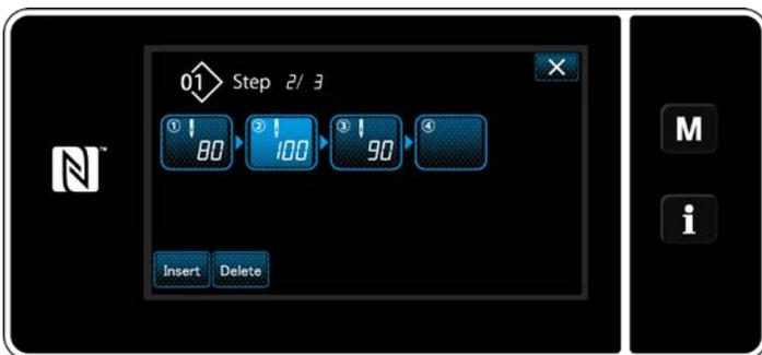
14) When **Delete** 17 is pressed, the selected step is deleted.
