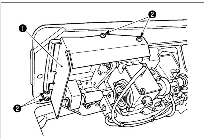
Install oil shield 1, supplied with the unit, on the frame with screws 2.
