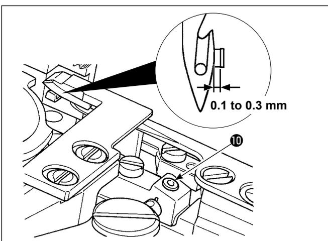
• **Adjusting the position of the bobbin thread clamp**
