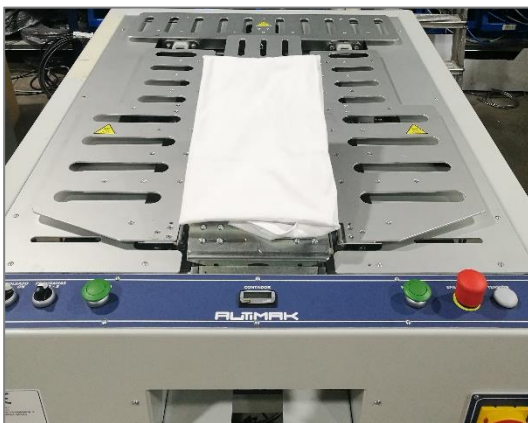
5) The horns go up (Bagging ON, it's also possible to deactivate it)
